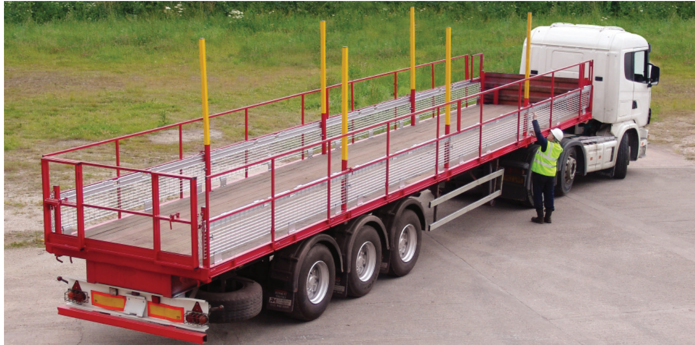
The trailer is prepared for unloading; The protective side panels are swung out and this allows the floor panels to be lowered into place.
