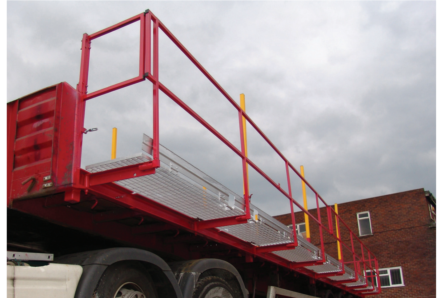
Safe access to the trailer is via a secured ladder. An operative may now safely move around the vehicle deck.
